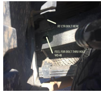
Figure 3 Right Center Bolt Lube Location
