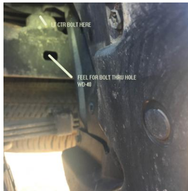
Figure 2 Left Center Bolt Lube Location
