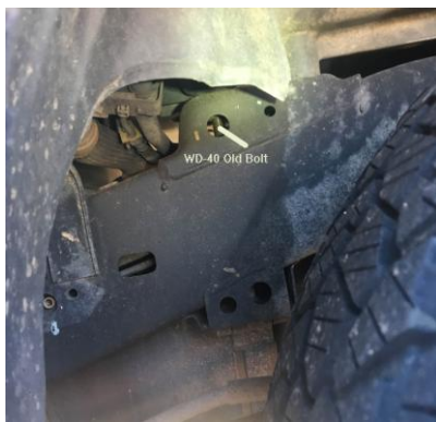
Figure 1 Left Front Bolt Lube Location
