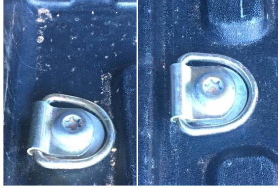
Figure 2 Mounted Front Left & Center Left (V-Ring Same)
